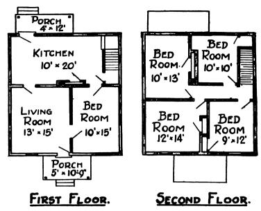
Fig. 42.—FIRST AND SECOND FLOOR PLANS OF DETACHED FRAME HOUSE FOR MINERS IN ANTHRACITE REGION,
